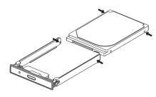
3. Slide mounting frame with HDD into the aluminium case
